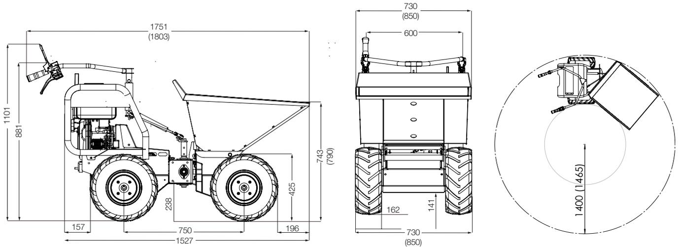
All dimensions unless otherwise stated are in millimetres. Dimensions B300 BENDie (B450 BENDie)
